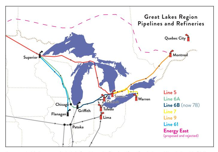
A vast network of pipelines serves refineries in the Great Lakes region. The rejected Energy East pipeline would have duplicated the Enbridge Great Lakes Line 5 short cut by transporting western Canadian oil to eastern Canadian refineries within Canada.
